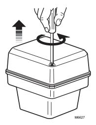
Fig. 4. Removing Actuator Cover.
