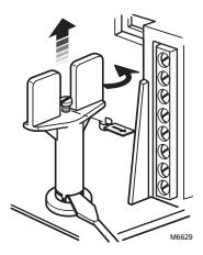
Fig. 5. Removing Spring Retaining Clip and Releasing Manual Spring Handle.
