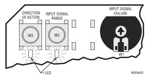
Fig. 15. Pushbuttons and potentiometer (default positions).
