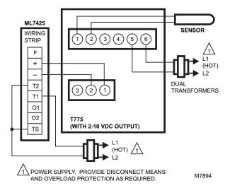
Fig. 10. ML7425 Wiring using 2 to 10 Vdc Control Signal and Separate Transformers.
