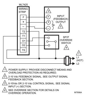
Fig. 16. Connections for Overriding Control Signal to Drive ML7425 to a Specific Position.
