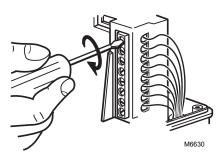
Fig. 6. Connecting Power and Control Wiring.
