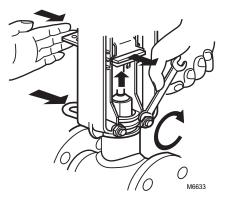
Fig. 3. Securing Actuator to Valve.
