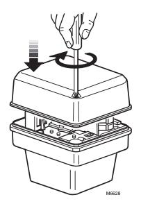
Fig. 14. Replacing Actuator Cover.
