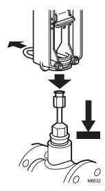
Fig. 2. Attaching Actuator to Valve Collar.
